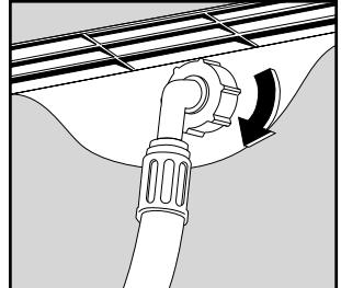
The other end of the inlet hose which connects to the machine can be turned in any direction. Simply loosen the fitting, rotate the hose and retighten the fitting, making sure there are no water leaks.
